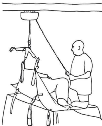
Repositioning sling attached to a lift hanger bar and used to turn a healthcare recipient on an exam table
