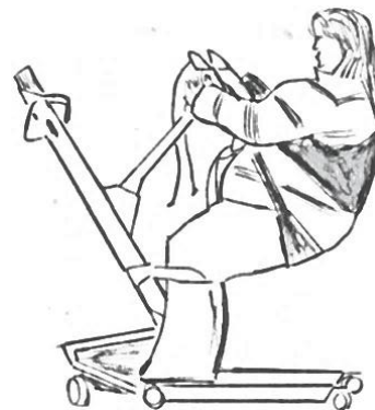
Sit-to-stand belt or sling with seat support attached to a powered sit-to-stand assist device using rope attachments supporting the health care recipient in the device
