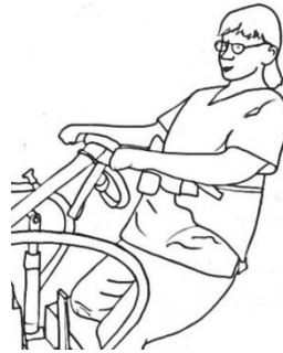
Sit-to-stand belt or sling attached to a powered sit-to-stand assist device and supporting the health care recipient in the device
